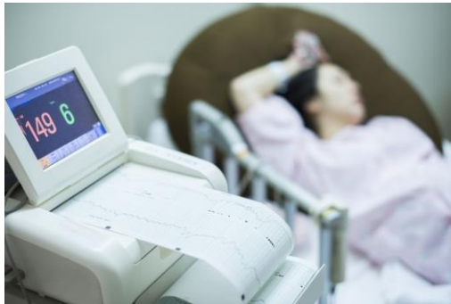
Processes uterine contraction and fetal heart rate data for remote monitoring of labor progress
